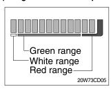
① This indicates the temperature of coolant.
